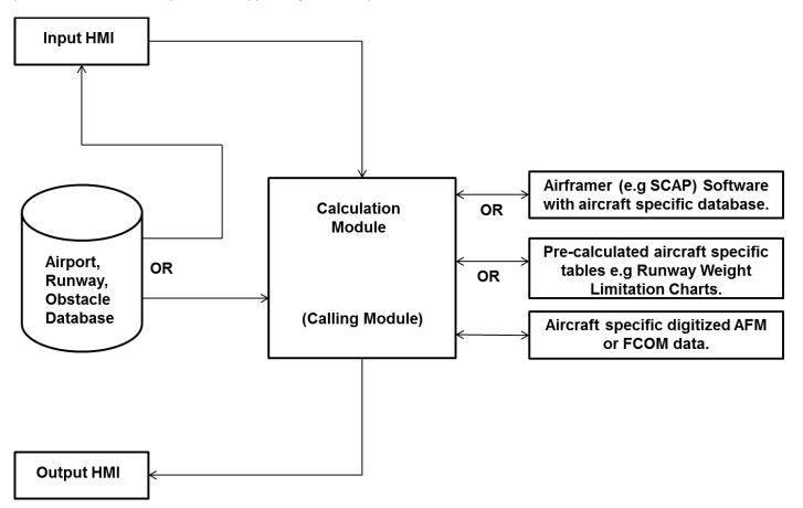
Figure 1. Typical architecture of a performance application
