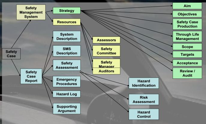
Figure 1. The Structure of a Safety Case.
